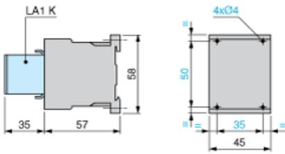
Contactors LC1 K, LP1 K, LP4 K: Mounting on Rail AM1 DP200 or AM1 DE200 (35 mm)
